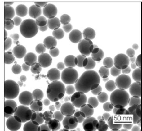
**Figure 7** Ultrafine fumed silica particles observed using TEM.<sup>37</sup> Courtesy Andri Vital, EMPA Mat's Testing & Research, Laboratory for High-Performance Ceramics, Duebendorf, Switzerland.
